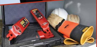
The PRX Proximity Voltage Detectors verify the presence of voltage without contacting the conductor. Three distinct models of testers have been developed for utility professionals:
