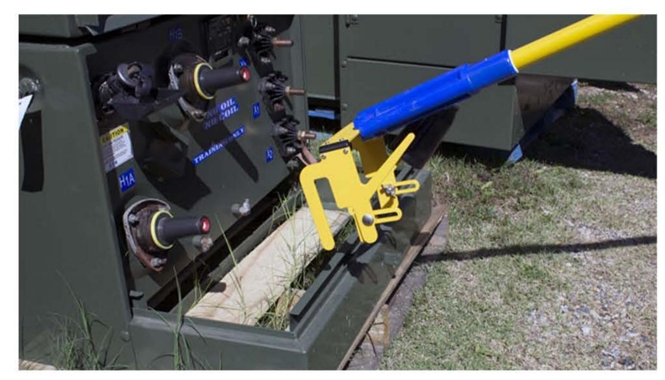
The patent-pending URD Cap Stand™ attaches to the lip of underground pad mount transformers and switchgear to securely hold insulated caps. It safely stores insulated caps that are accessible using a shotgun stick so workers remain outside their minimum approach distance (MAD) and caps stay clean.
